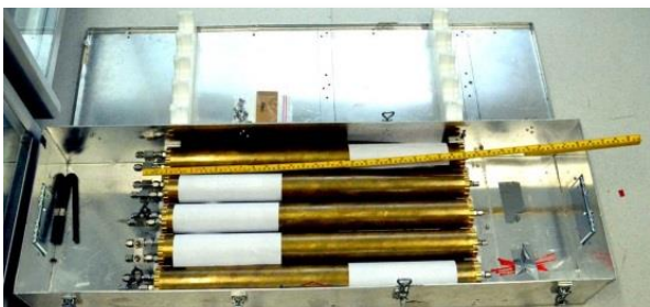
Fig. 2 Brass tubes with drillcores for analysis of gas in the rock matrix
