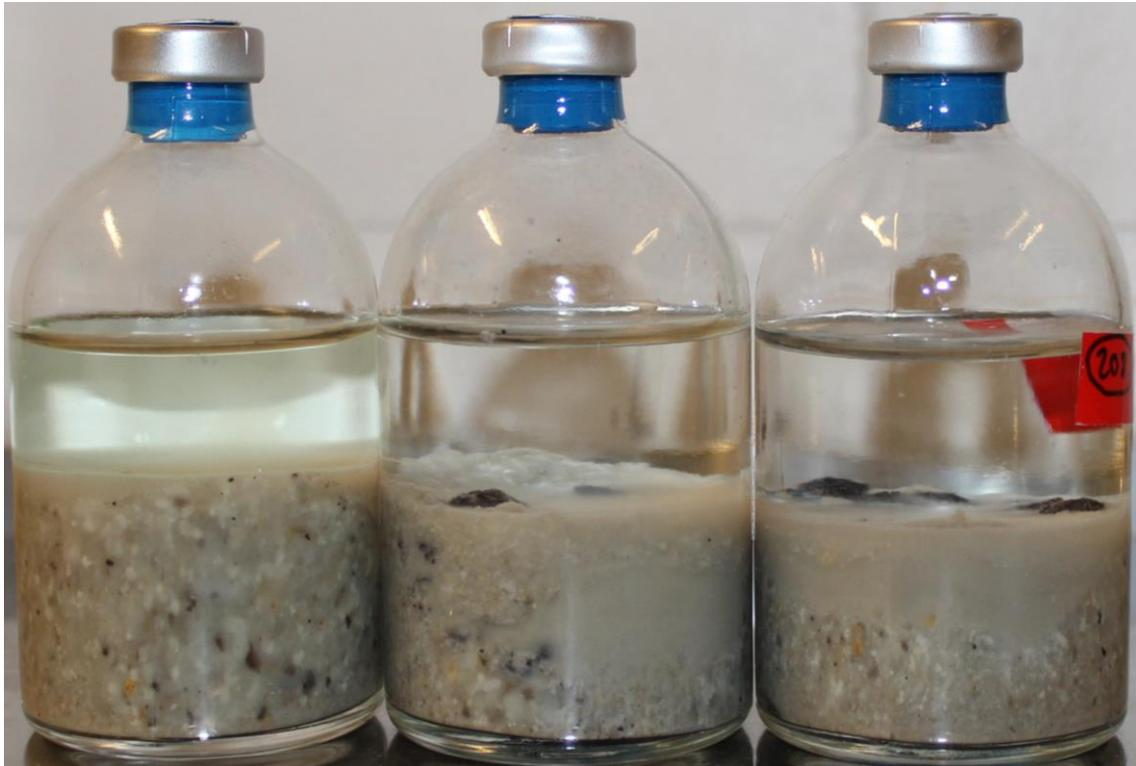
Figure 1-1. Bentonite storage bottles from left to right: Control 1, Control 2 and Test bottle.
