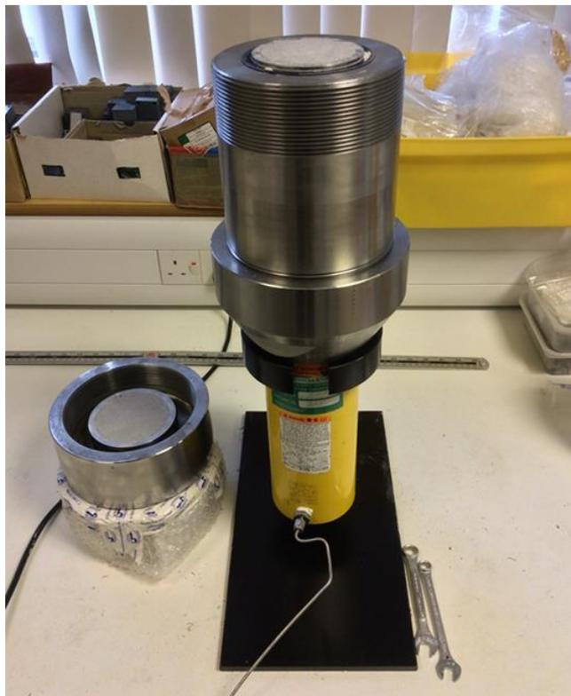
Figure 2-2. Press used to compress the samples to the required density.
